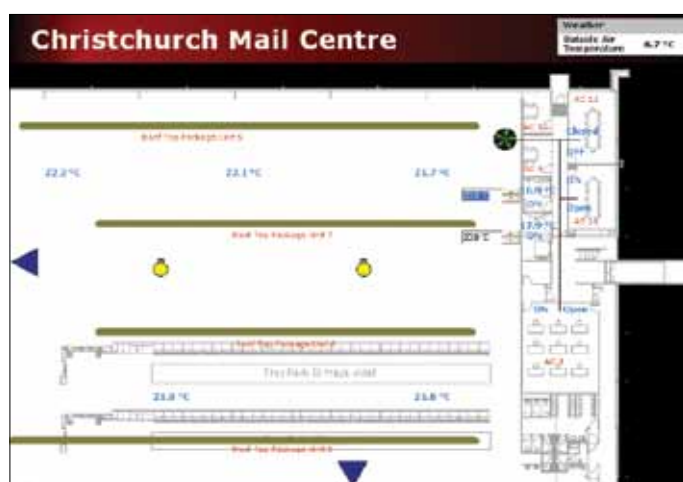
New Zealand Post Mail centre BMS © Copyright
